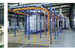
Automatic frame powder spraying production line
